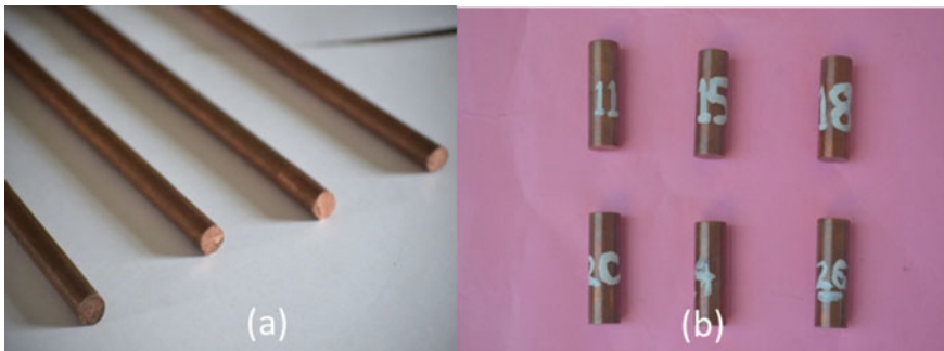
Fig. 5 a Raw copper rod and b copper electrode after machining
