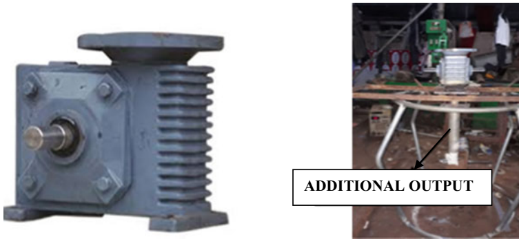
Fig. 1 Regular gearbox (left) and modified gearbox (right) with vertical output
