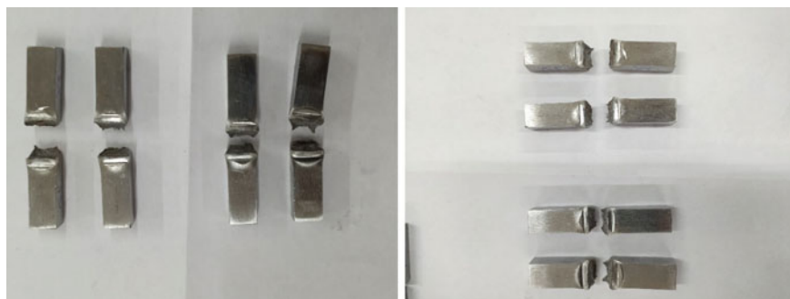
Fig. 8 Fractured Charpy samples of X and Y directions
