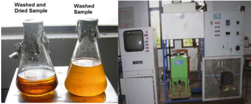
Fig. 2 Final washed sample of Karanja Bio-Diesel along with experimental setup
