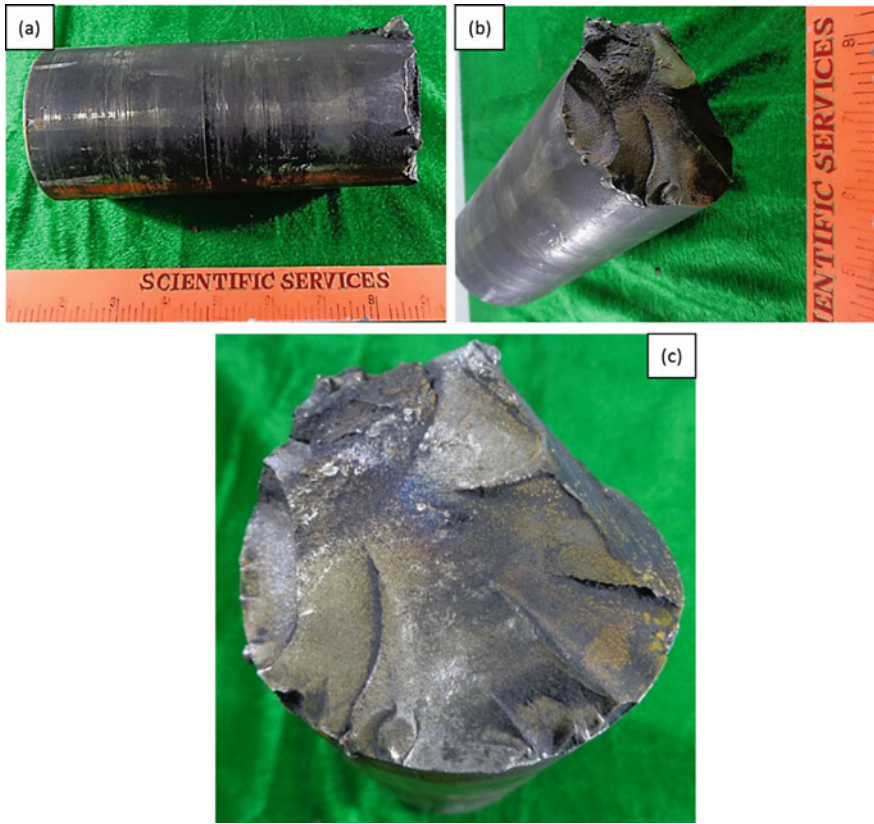
Fig. 6 Visual images of failed bend pulley: a bend pulley along its length, b angular view of the shaft, c fracture surface revealing multiple ratchet marks
