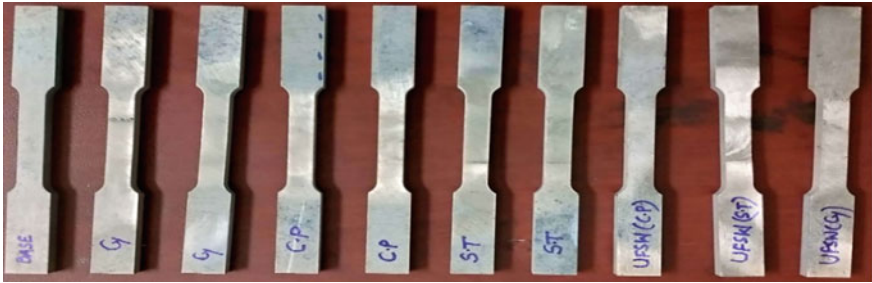
Fig. 10 Tensile test specimens for air and underwater
