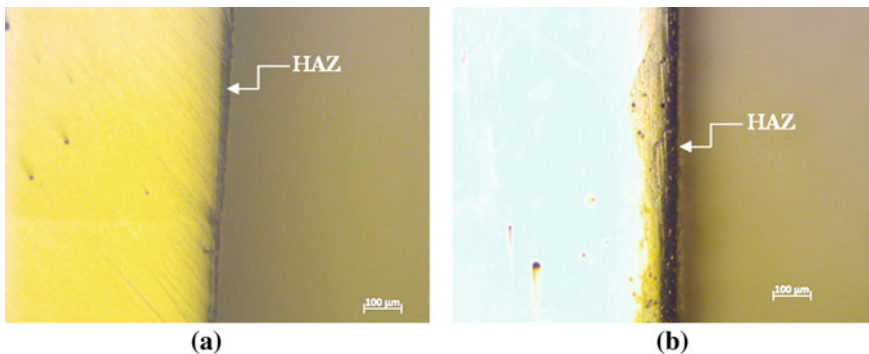
Fig. 7 Macrograph of the samples at 100X observed to measure HAZ thickness a 50% SS304L + 50% Inconel 625 samples machined at 2 µs, and b 100% Inconel 625 samples machined at 5 µs
