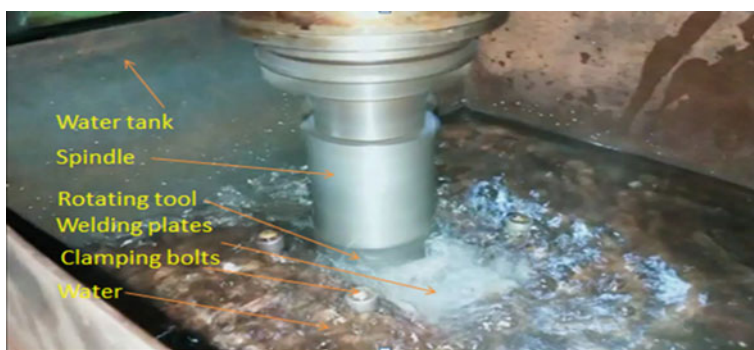
Fig. 5 Underwater FSW process
