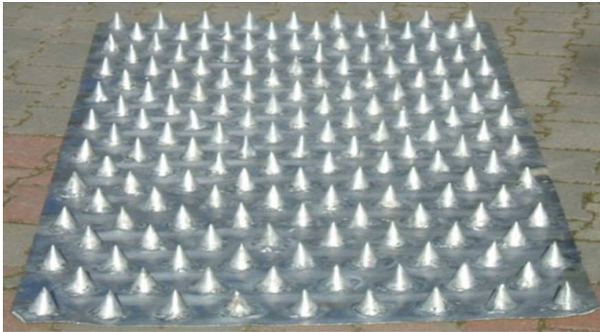
Fig. 10 Absorber plate with conical surfaces [10]
