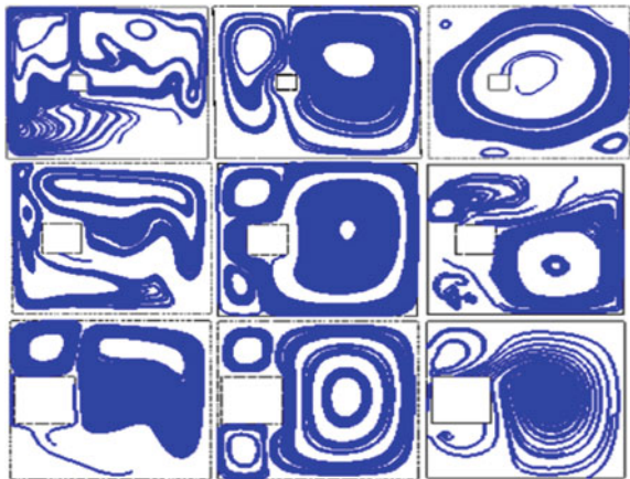
Fig. 3 Isotherms of natural convective flow for working fluid air, water, and nanofluid for Ra = 10^5 for a single plate allocated internally in a square enclosure at x_c = 0.15, 0.25, and 0.35 respectively
