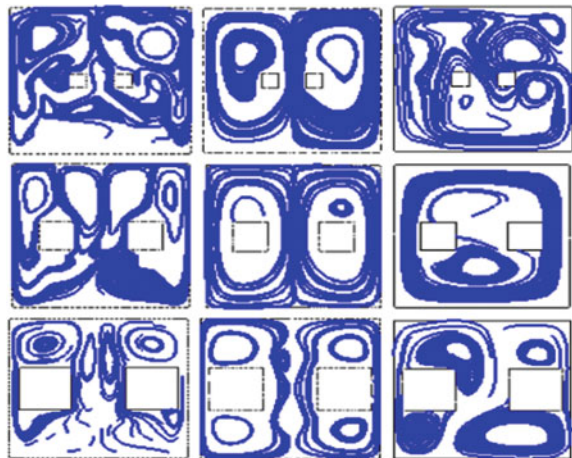
Fig. 6 Isotherms of natural convective flow for working fluid air, water, and nanofluid for Ra = 10^5 for a pair of plate allocated internally in a square enclosure at \delta = 0.3 , 0.5 and 0.6 respectively
