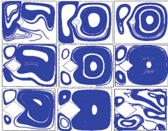
Fig. 8 Isotherms of natural convective flow for working fluid air, water, and nanofluid for Ra = 10^4 for a single tilt plate allocated internally in a square enclosure at x_c = 0.15, 0.25, and 0.35 respectively
