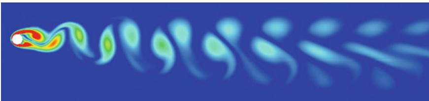
Fig. 10 Vortex structure at Ri = -1 on the bottom surface and Re = 100 . Shedding is not symmetric to the horizontal axis due to cooling
