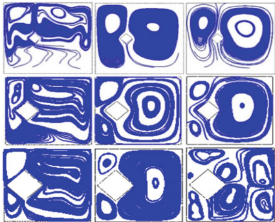
Fig. 9 Isotherms of natural convective flow for working fluid air, water, and nanofluid for Ra = 10^5 for a single tilt plate allocated internally in a square enclosure at x_c = 0.15, 0.25, and 0.35 respectively
