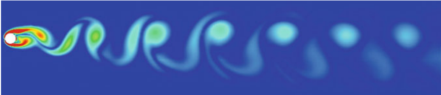
Fig. 9 Vortex structure at Ri = -1 on the top surface and Re = 100 . Shedding is not symmetric to the horizontal axis due to cooling
