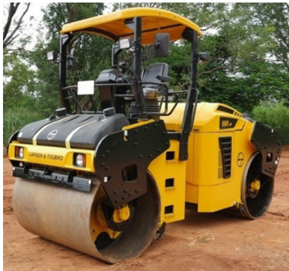
Fig. 76.1 Vibratory tandem compactor
