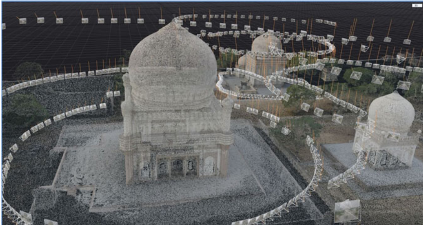
Fig. 62.3 Sparse point clouds for four of the tombs generated in reality capture
