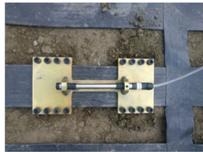
Fig. 7 Fixing the strain gauges with plates on primary reinforcement (geogrid) at the site for valley side reinforced soil system
