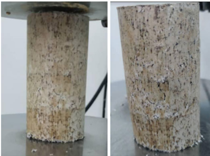
Fig. 8 UCT of 80:20 mixtures (before and after the test)
