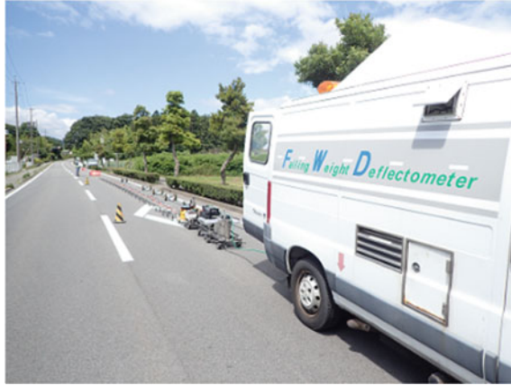
Photo 4 FWD vehicle towing the carrying carts for accelerometers and electric resistivity logging system
