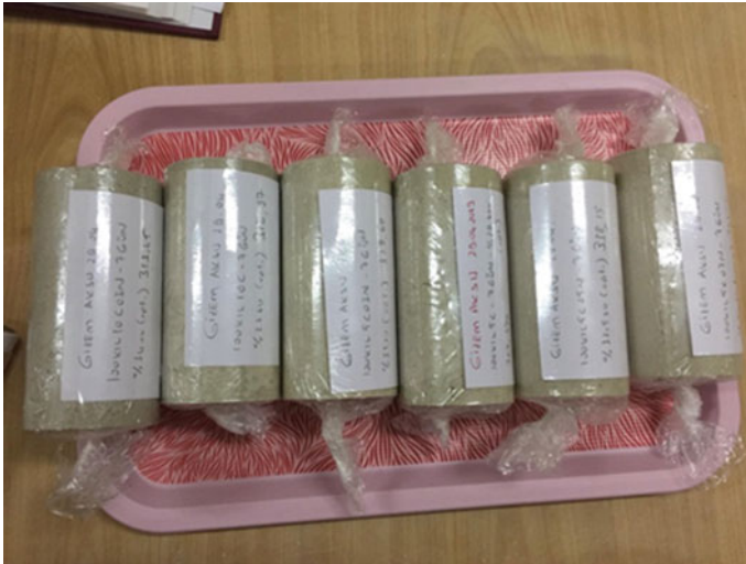
Fig. 1 Cement and/or nanosilica admixed clay specimens with a curing period of 7 days
