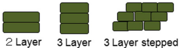
Fig. 8 Different condition of tire placement for WFT
