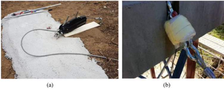
Fig. 5 a Pulling hoist clamped on the counterweight and b the load cell attached to the roof slab
