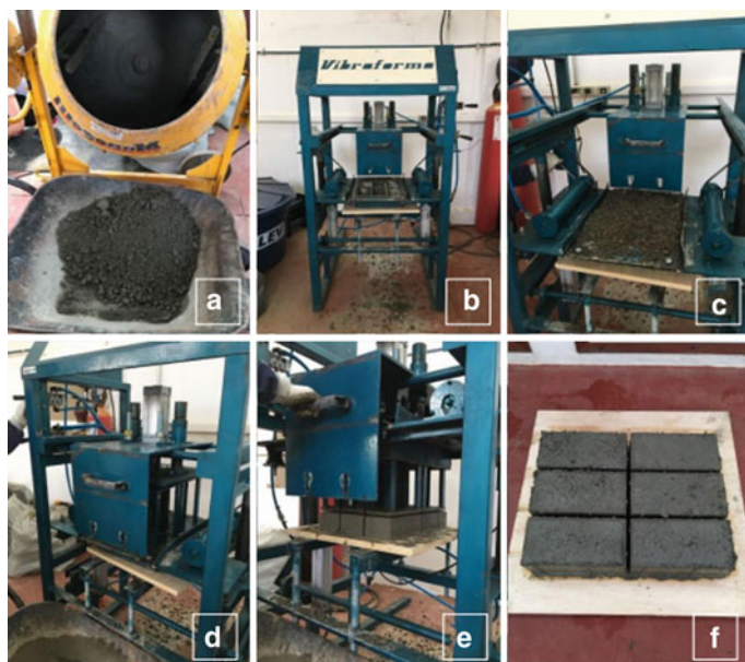
Fig. 1 Process of manufacturing of blocks with mining waste [7]
