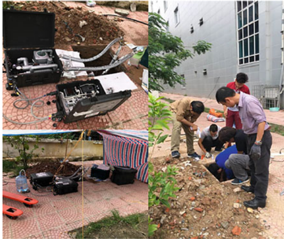
Fig. 19 TRT measurement in the GSHP site at VIGMR, Hanoi
