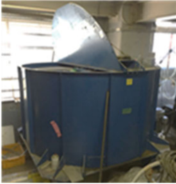
1) Outside of small centrifugal model experiment device
