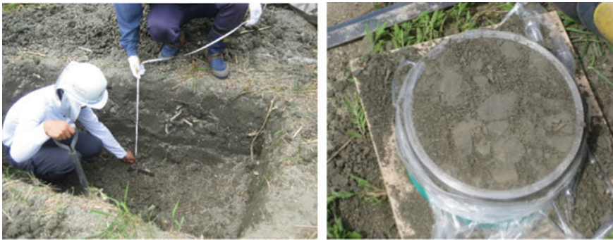
Fig. 12 Situation of the dike and a block sample taken near No. 9 in 2017
