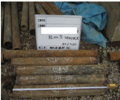
(c). Cut piles.
