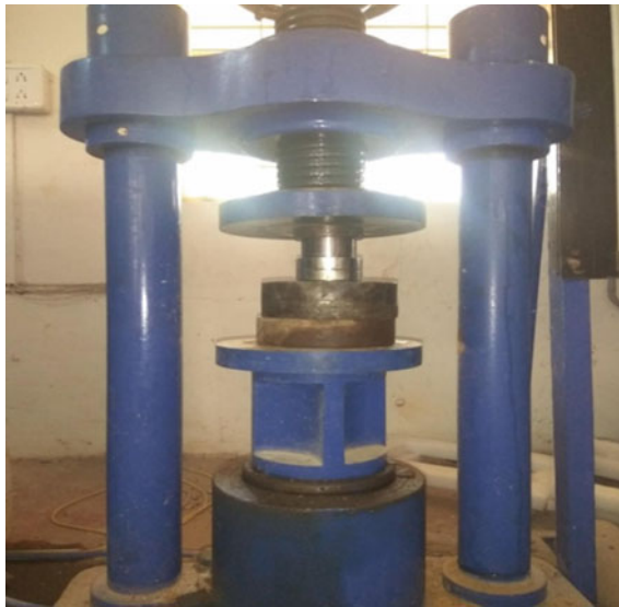
Fig. 3 Oedometer mold placed in UTM
