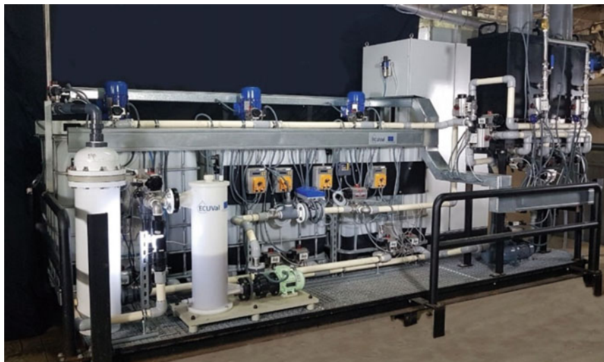
Fig. 7 EC-UV industrial system currently operating in a mill for the treatment of coloured and saline effluents at 4 m 3 /h
