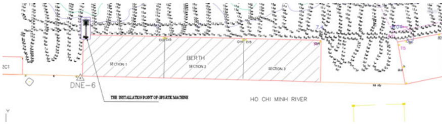
Fig. 2 The selected location for installing automatic monitoring equipment
