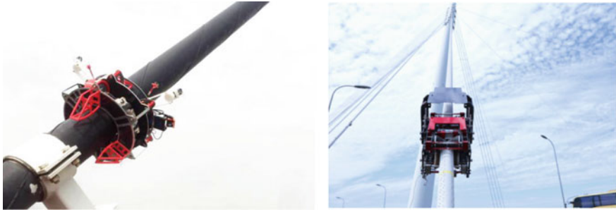
Fig. 1 Cable inspection robot
