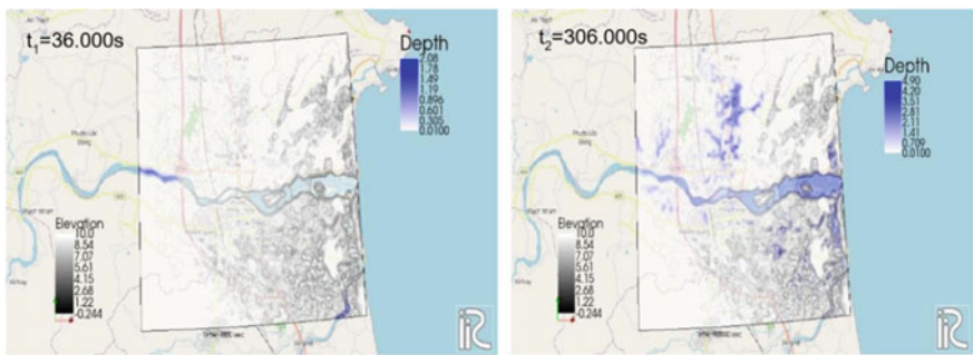
Fig. 4 Computed inundation map of Tra Khuc's downstream at two time instances
