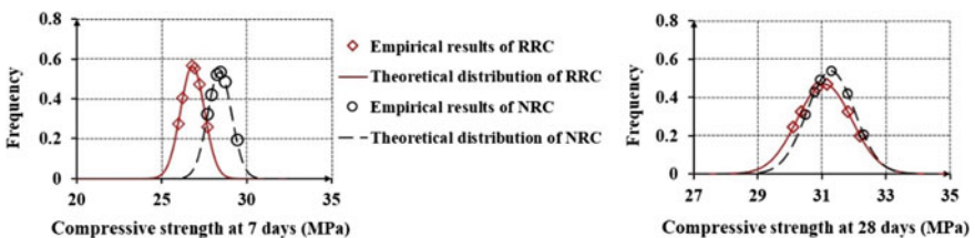
Fig. 1 Frequency and equivalent theoretical distribution curves of the empirical compressive strengths at 7 and 28 days age of two designed lining concretes
