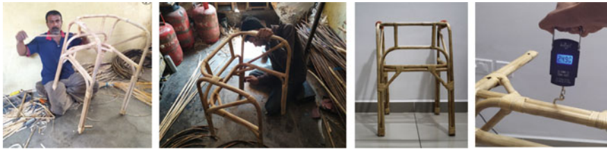
Fig. 15.7 Process of walker design using rattan cane
