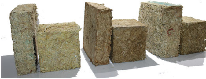
Fig. 69.7 Bio-bricks sizes—(150 × 150 × 50 mm) and (100 × 100 × 100 mm)
