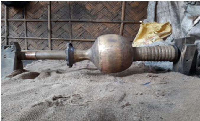
Fig. 22.1 Existing Kalash polishing tool
