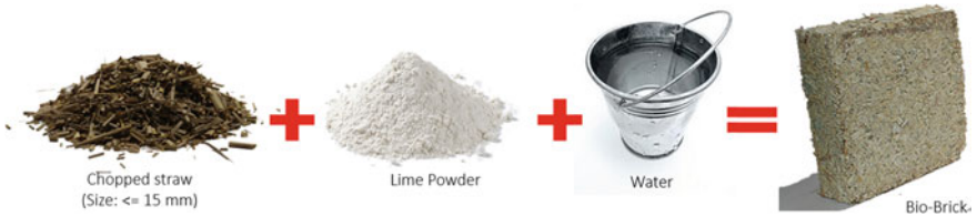
Fig. 69.5 Process of making bio-bricks
