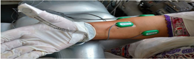
Fig. 3.3 Placement of the flexi force sensor on the thumb tip
