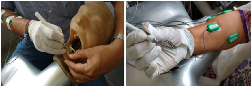
Fig. 3.2 Dental scaling task being performed on typodont and EMG electrodes placed on upper extremity and flexi force sensors on gloves
