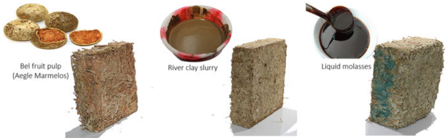
Fig. 69.6 Different natural binders added to the bio-bricks mixture
