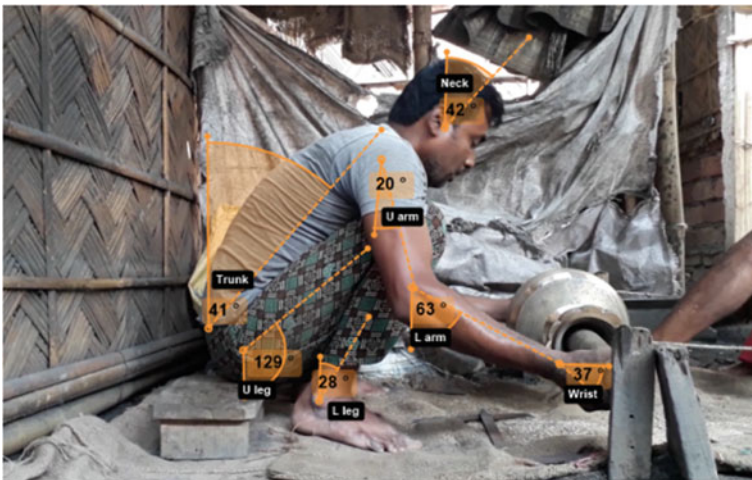
Fig. 22.4 Joint angle detection of the polisher
