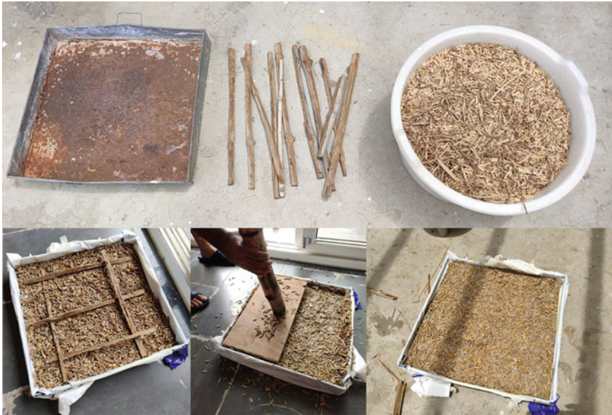
Fig. 69.14 Making of the insulation panel
