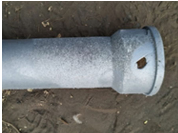
Fig. 6 Casting defect due to misrun
