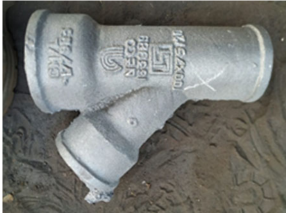
Fig. 7 Defected casting due to slag inclusion
