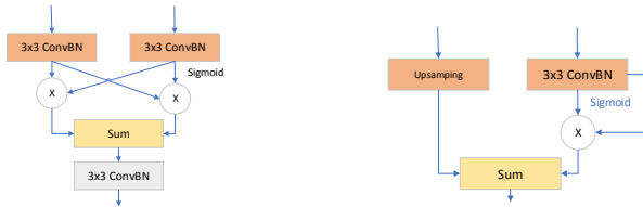
(a) Feature Extraction and Fusion Module (FEFM), (b) Small Feature Extraction and Fusion Module (SFEFM)
