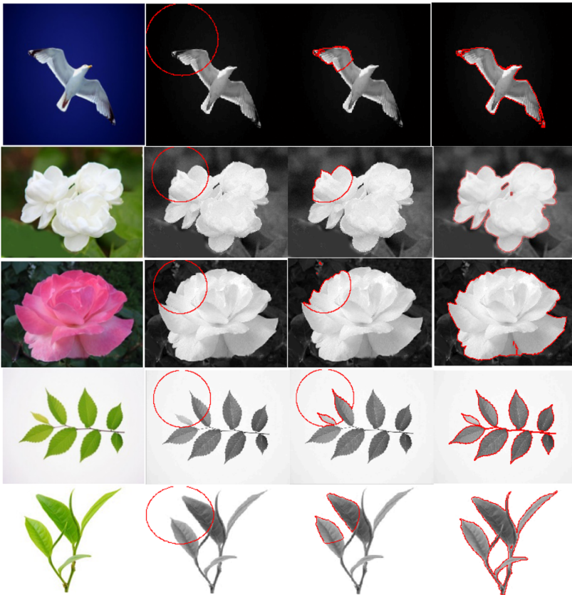
Fig. 3. Segmentation results on real images with slight complex background. The first column is given images; the second column is the initial contours; the third column is the results of the first iteration of sweeping; the forth column is results of the final segmentation.
