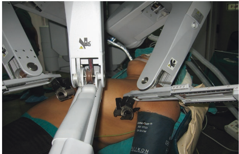
Fig. 19.3 The robot docking covers the patient's torso and head, limiting access to the airways of the patient
