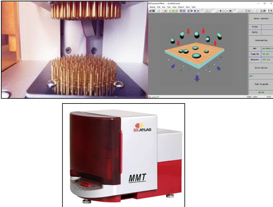
Fig. 6 Top and bottom sensors of moisture management tester
