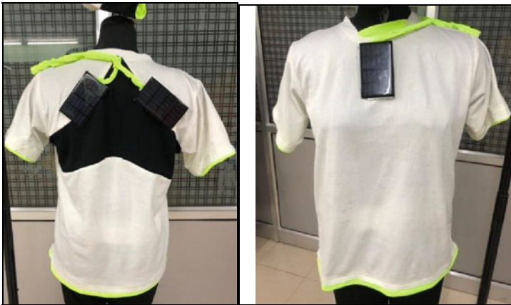
Fig. 12 Solar panel integrated t-shirt
