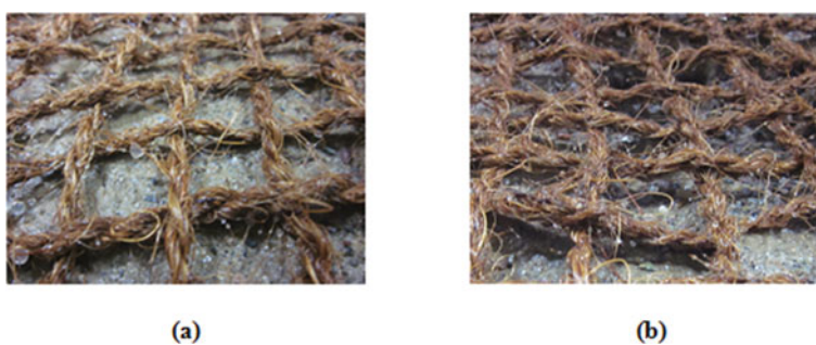
Fig. 5 Drapability of coir RECSs at different slope angle: a sheet erosion and lower slope angle; b gully erosion at steeper slope angle
