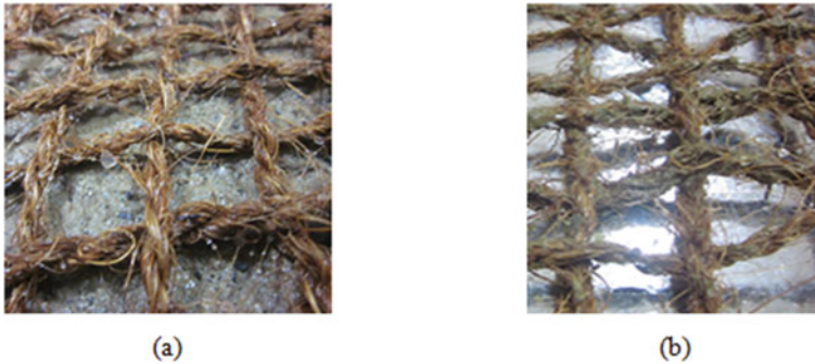
Fig. 7 Coir RECSs laid at different infiltration condition: a soil infiltration condition (soil trays); b zero-infiltration condition (metallic ramp)
