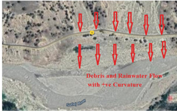
Fig. 8 Positive curvature of landslide
