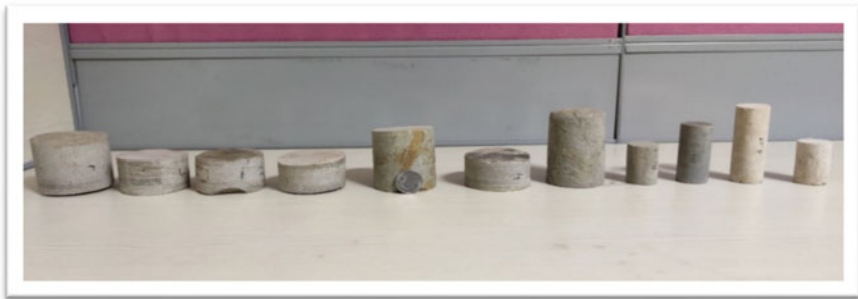
Fig. 2 Core samples collected for performing ultrasonic pulse velocimetry measurement (A1 to A11 from left to right)
