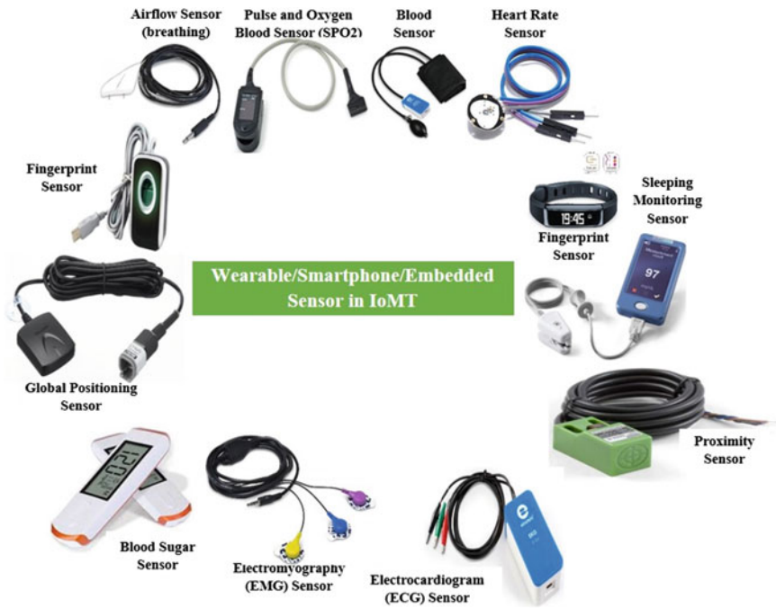
Fig. 3 Sensor devices for collection data on IoMT
