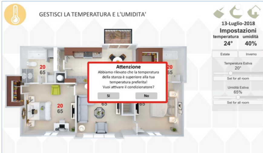
Fig. 8 The DEA alerts the resident that detected temperature is outside his/her comfort range and asks him/her whether he/she wants to activate the air-conditioning system
