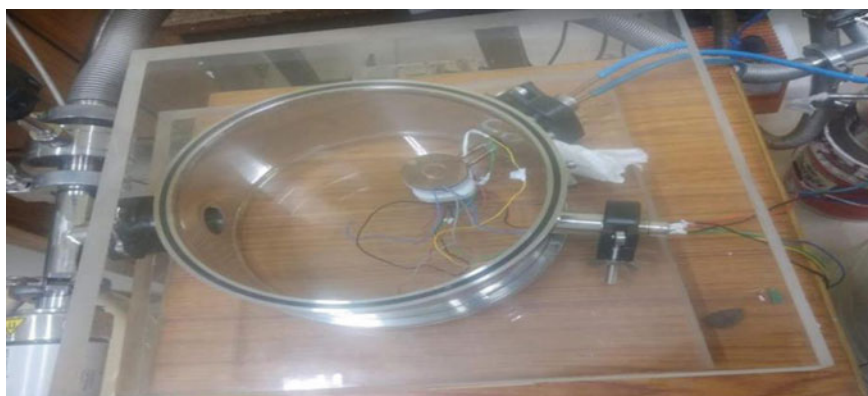
Fig. 27 Base 3 connected to KF16 connector in perplex setup
