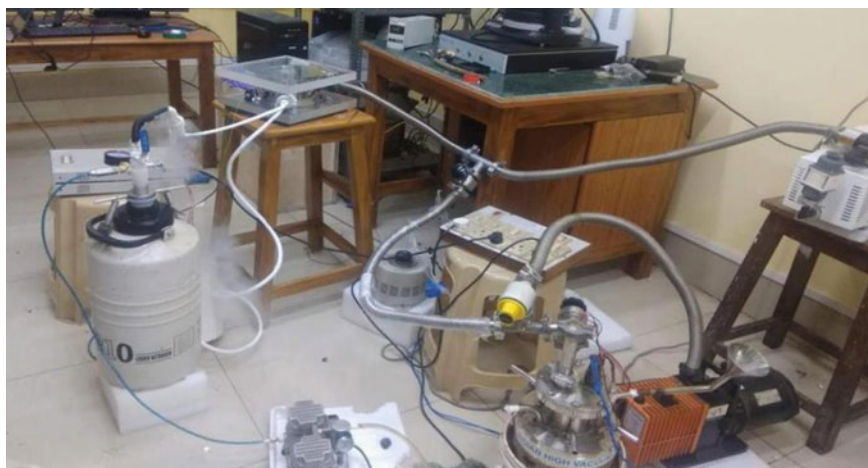
Fig. 25 Vacuum system connected to cylindrical hood through KF25
