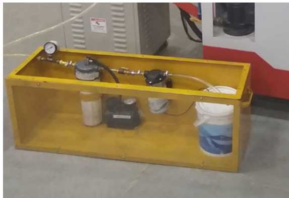
Fig. 1 Fabricated portable mist lubricator setup (PMLS)
