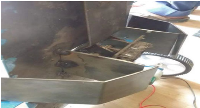
Fig. 7 Fabrication of holding arms
