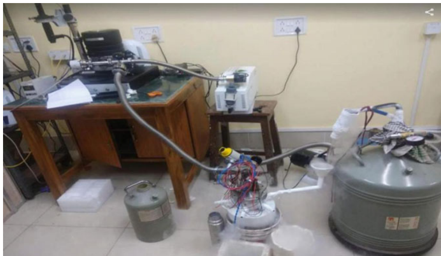
Fig. 26 Vacuum system connected to main AFM
