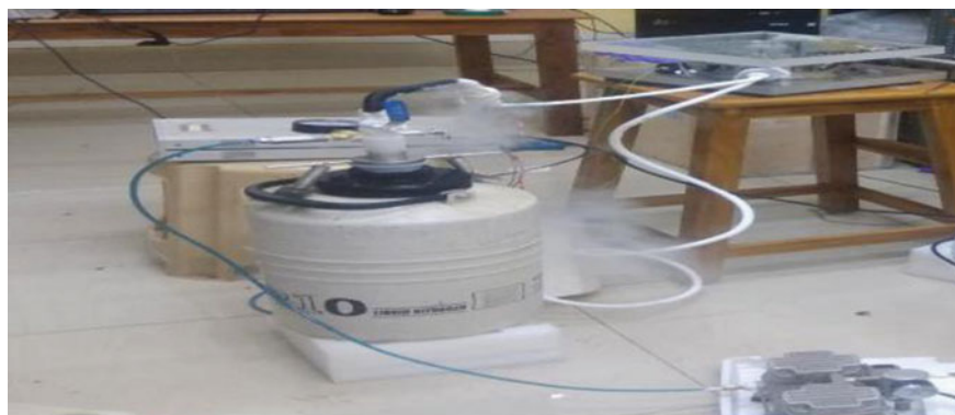
Fig. 21 Transfer device connected to perflex setup
