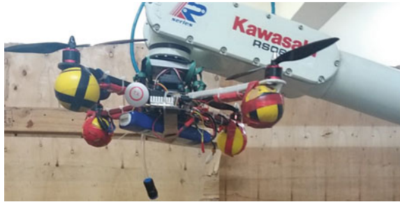
Fig. 1 Quad copter fixed to the Kawasaki 6 DoF robot
