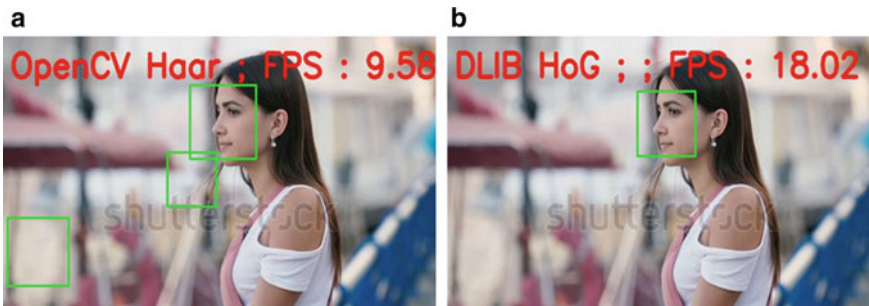
Fig. 9 a OpenCV haar, b Dlib HoG implementation example 2
