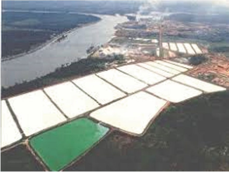
Fig. 12.2 Settling ponds for kaolin tailings. (Source: Barata et al. (2008))
