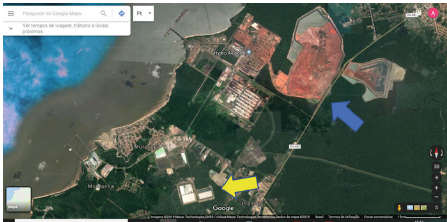
Fig. 12.3 Satellite view (Google Maps) of the municipality of Barcarena, State of Pará-Brazil, where one can see settling ponds for tailings from the kaolin industry (yellow arrow) and “red mud” from aluminum (blue arrow)
