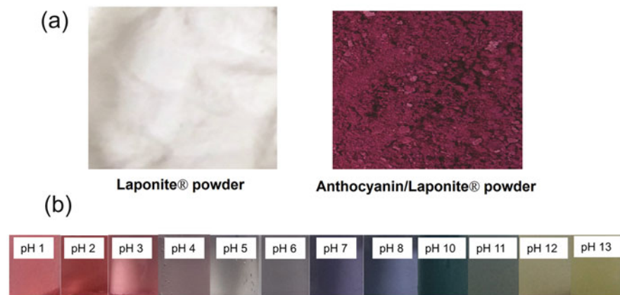
Fig. 5.2 (a) Laponite® powder and anthocyanin/laponite® powder and (b) color changes of anthocyanin/laponite® powder as a function of pH. (Source: Adapted with permission from Capello et al. (2019))
