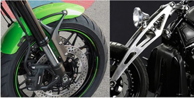
Fig. 1 Telescopic fork versus girder fork [1, 2]
