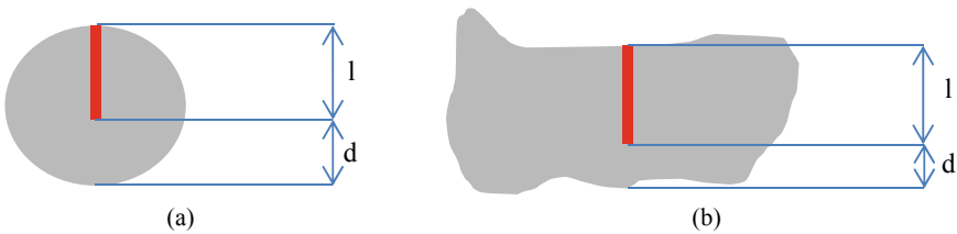
Fig. 8 Estimations of air-pocket thickness: a spherical pocket; b distorted pocket
