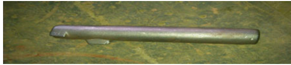
Fig. 1 Photograph of sand casted part of spheroidal graphite iron
