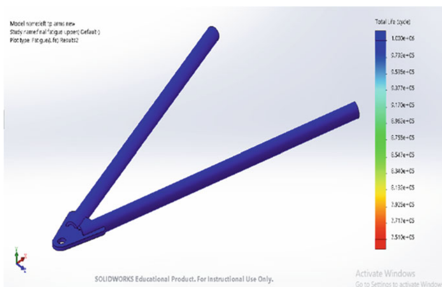
Fig. 14 Fatigue stress simulation of upper control arm
