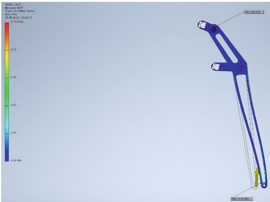
Fig. 7 Von-Mises stress distribution. Maximum stress 11.53 MPa
