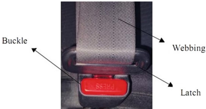
Fig. 1 Existing seat belt locking system (Maruti Wagon R)
