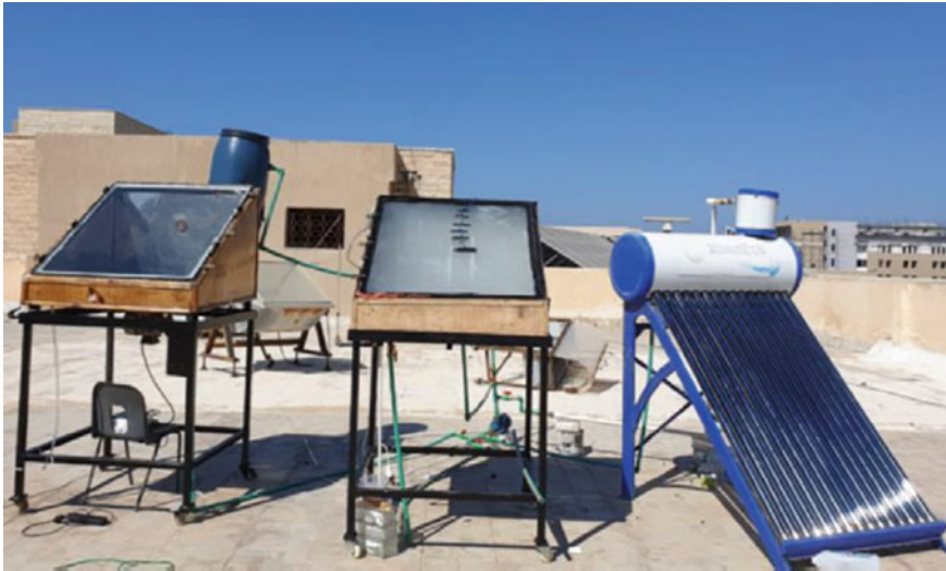
Fig. 9 Photograph of solar still with and without ETC [32]
