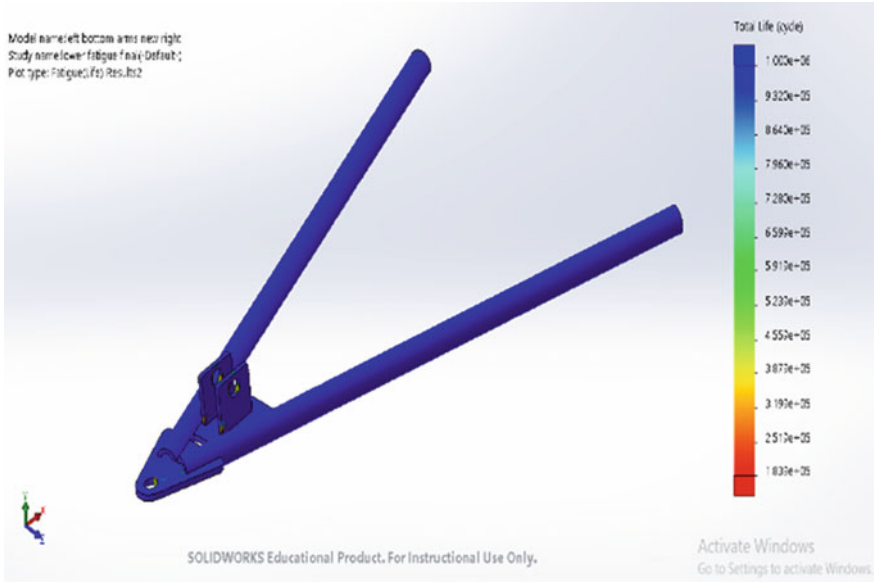
Fig. 15 Fatigue stress simulation of lower control arm
