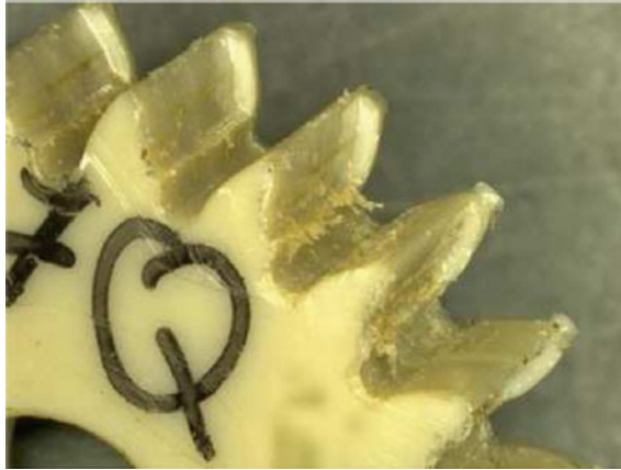
Fig. 4 PEEK-gear wear during operation with no added lubrication at torque 1.0 Nm, rotational speed 1600 rpm, wear after 9.13 \times 10^6 cycles (Reproduced with permission of Zorko et al. 2019)
