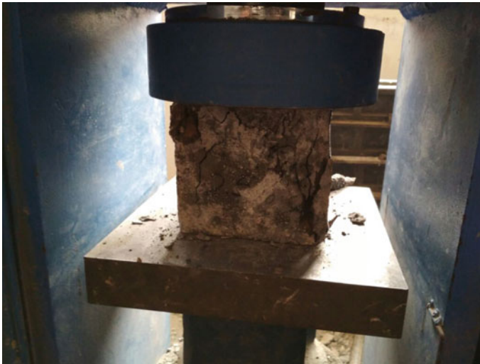
Fig. 3 Compression strength test of M20
