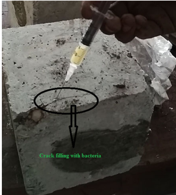
Fig. 6 Addition of bacteria along with its food into the cracks for self-healing action
