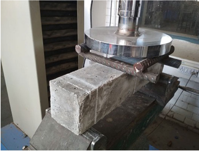
Fig. 4 Flexural testing of specimen
