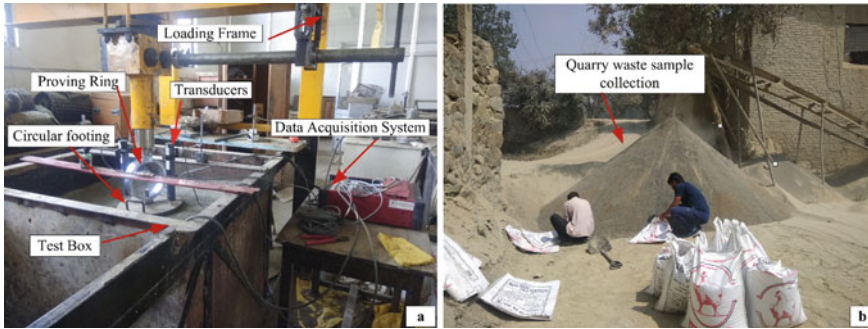
Fig. 1 Showing test setup and quarry waste material collection
