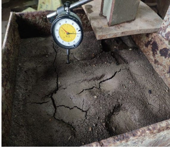
Fig. 12 Complete saturation of soil without GPA
