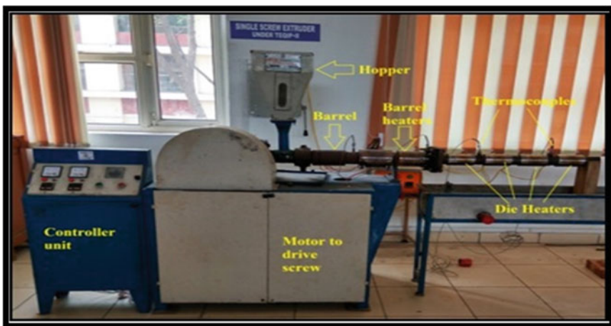
Fig. 3 Single-screw extruder
