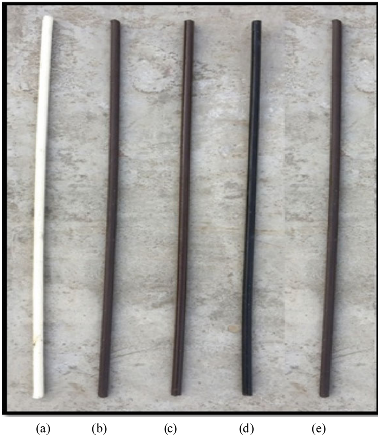
Fig. 4 Developed rods a pure PLA; b 10% fiber fraction; c 20% fiber fraction; d 30% fiber fraction; e 40% fiber fraction
