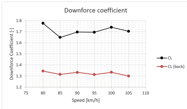
Fig. 4. Downforce coefficient of the car in both directions. (wind speed was about 5km/h)
