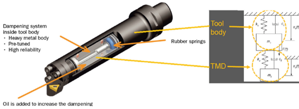
Fig. 2. Tuned mass damper (Silent Tool – Sandvik) and dynamic model [22].
