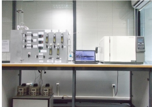
Fig. 10. Synthetic gas bench of oxygen reduction system and gas chromatography analyser.
