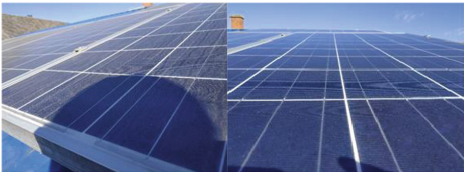
Fig. 6. The ninth day was dirty solar panel (left) and post-rain solar panel (right).
