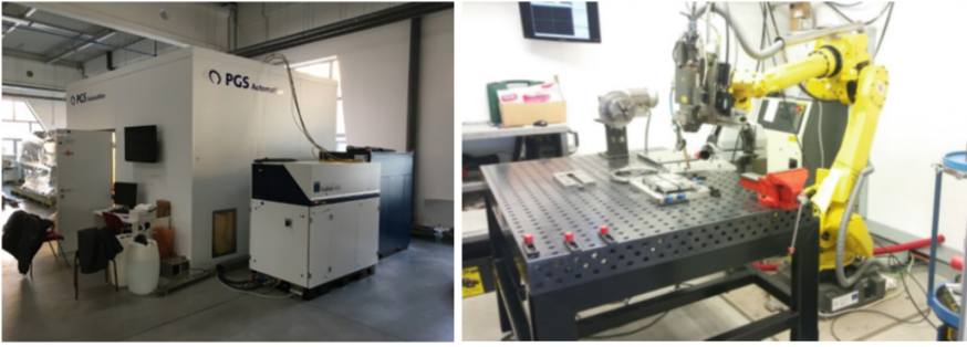
Fig. 1. Laser welding equipment and Fanuc Robot M-710 iC50.
