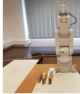
Fig. 5. Pick and place scenario by RV-2AJ arm.
