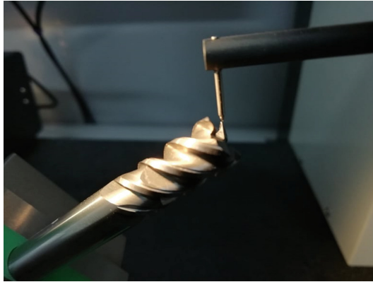
Fig. 4. Touch measurement of the tool's cutting edge on ZEISS Surfcom 5000
