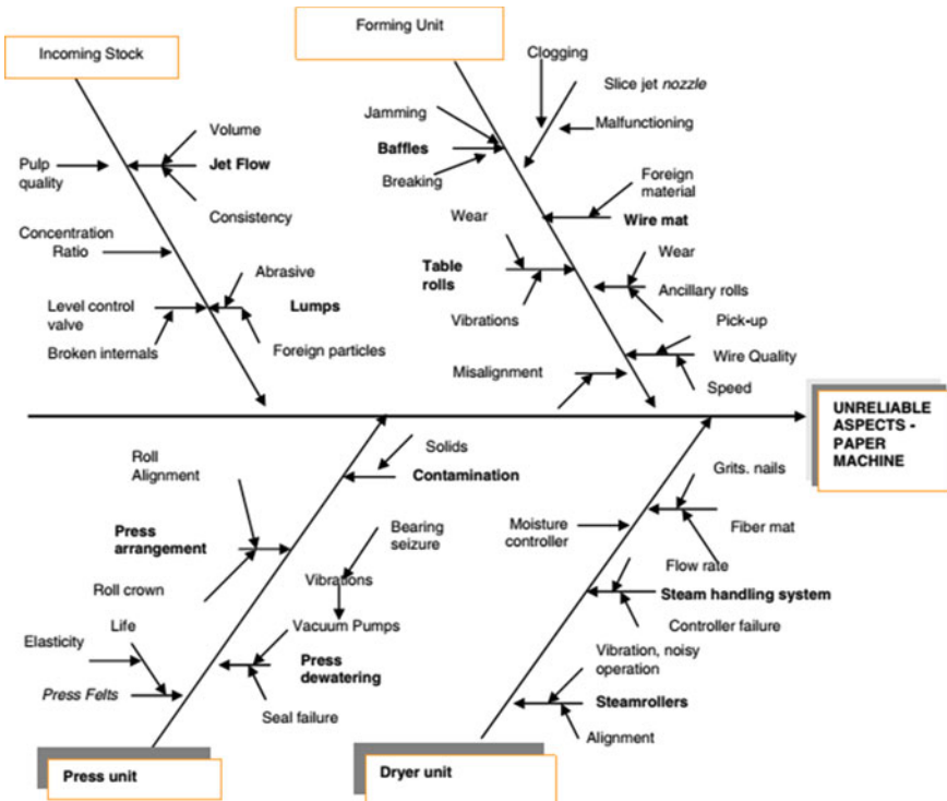
Fig. A.6. Cause and effect diagram
