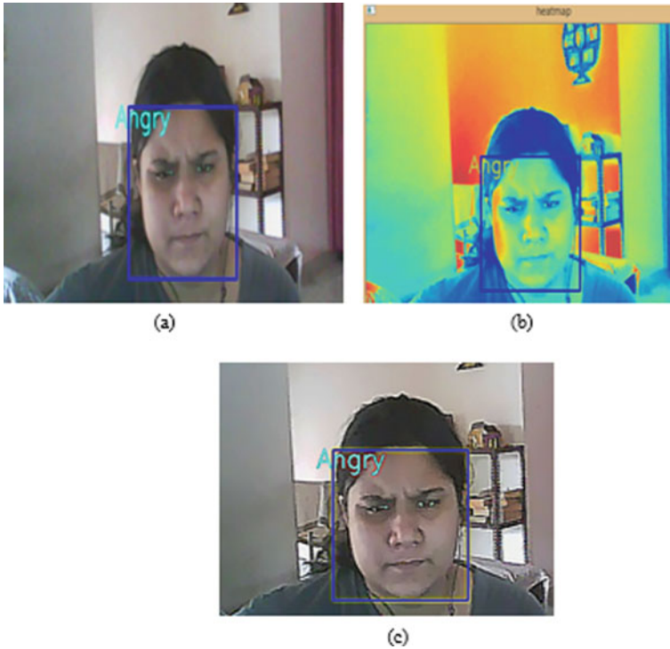
Fig. 7 Video pre-processing a input frame, b heatmap and c frame after pre-processing
