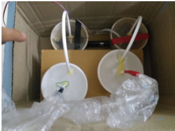
Fig. 18 Electrolysis process of the oxygen generator (red colour specifies oxygen and black colour specifies hydrogen)
