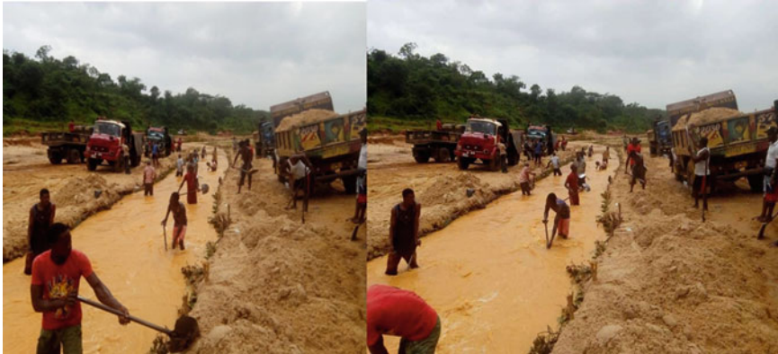
Plate 16.1 Miners extracting huge volumes of sand from the riverbed using shovels and transferring the sands into the trucks. It also showed the knee/ankle-depth level of the river, indicating river alteration, width reduction, and change in river channel network
