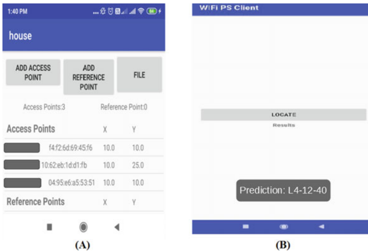
Fig. 3 a Android application for data collection b Client side location query application showing the predicted location
