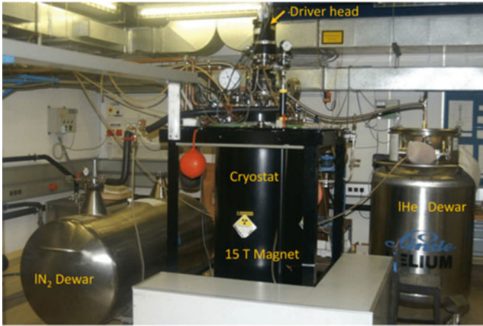
Fig. 8.12 15 T high field Mössbauer equipment at the Institute of Solid State Physics, TU Wien, Austria
