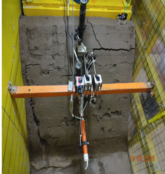
Fig. 12 Failure mechanism of the slope after imposing rainfall, static stress, and dynamic condition
