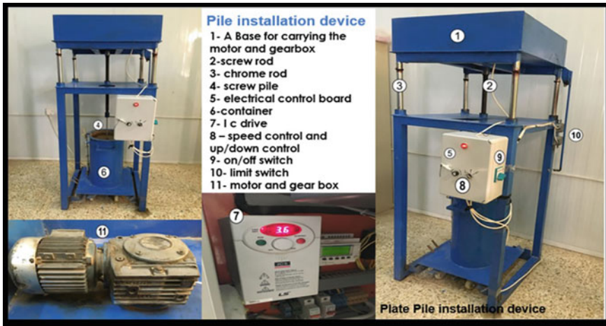
Fig. 4 Hydraulic torque motor (screw pile installation device)
