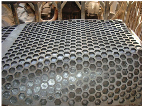
Fig. 7 The manufactured mesh of honeycombed type
