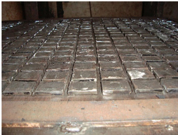
Fig. 2 Metal mold for mesh with rectangular openings
