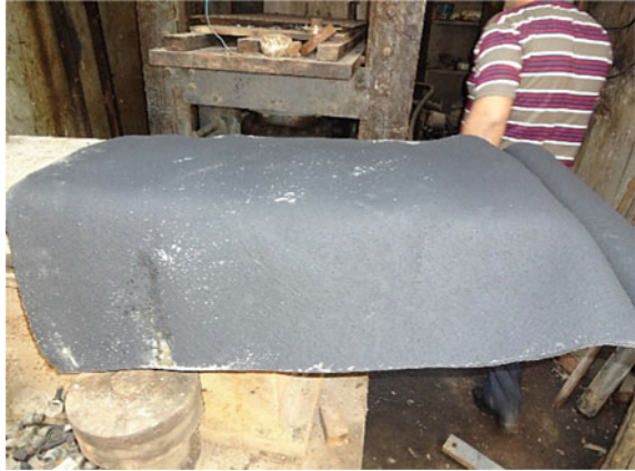
Fig. 3 The raw rubber used in manufacturing geogrids
