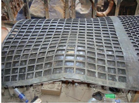
Fig. 8 The manufactured geogrid mesh of rectangular openings
