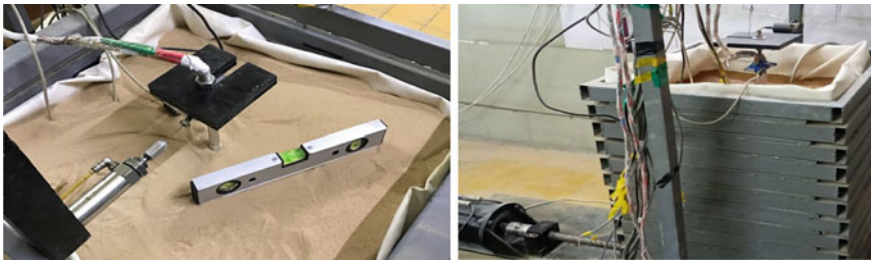
Fig. 1 Shaking table box with complete setup
