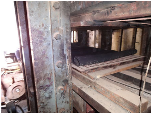
Fig. 5 The raw rubber placed in the metallic mold before applying temperature
