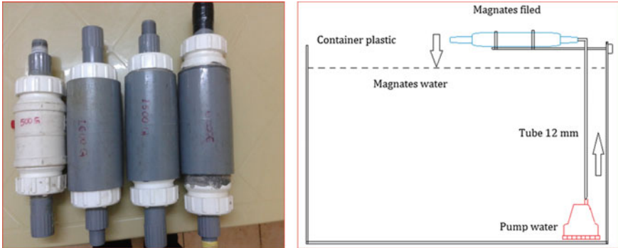
Fig. 2 Devices of magnetic fields and preparation of magnetic water
