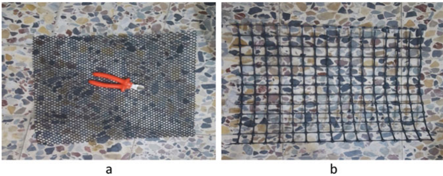
Fig. 4 The two types of geogrids used; a: Netlon CE121 b: Tensar SS2
