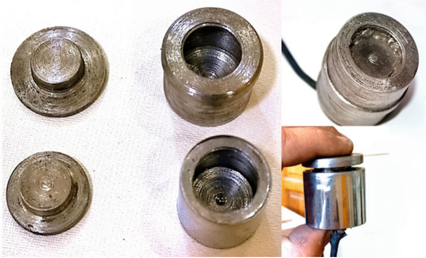
Fig. 5 Types of the steel container of load cells to measure end bearing resistance
