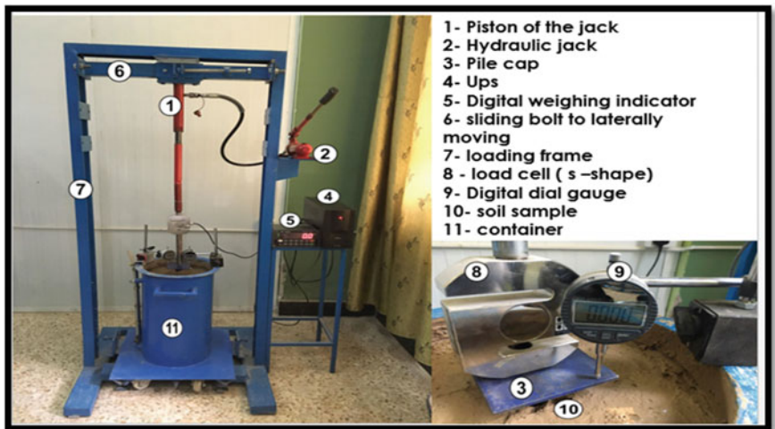
Fig. 5 Pile test device
