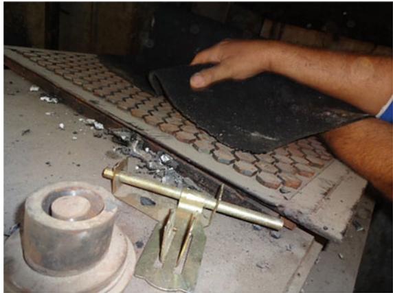
Fig. 4 Placing of rubber in the metallic mold
