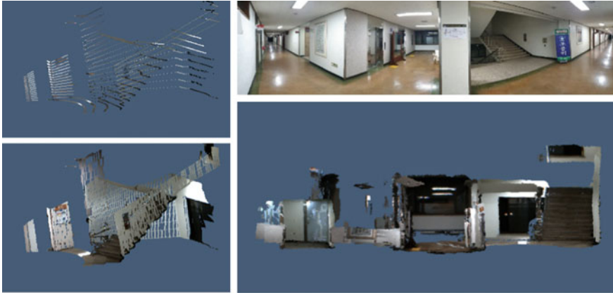
Fig. 7 Depth upsampling result (left) and 3D map building result (right)
