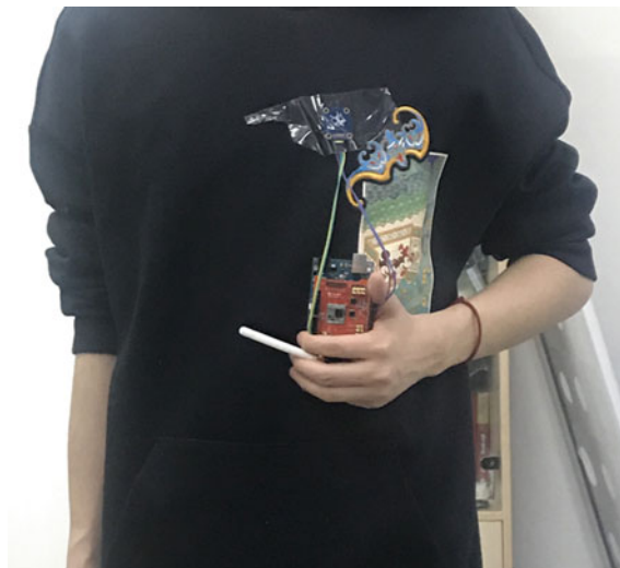
Fig. 2 Terminal device carried on experimenter to detect real-time posture
