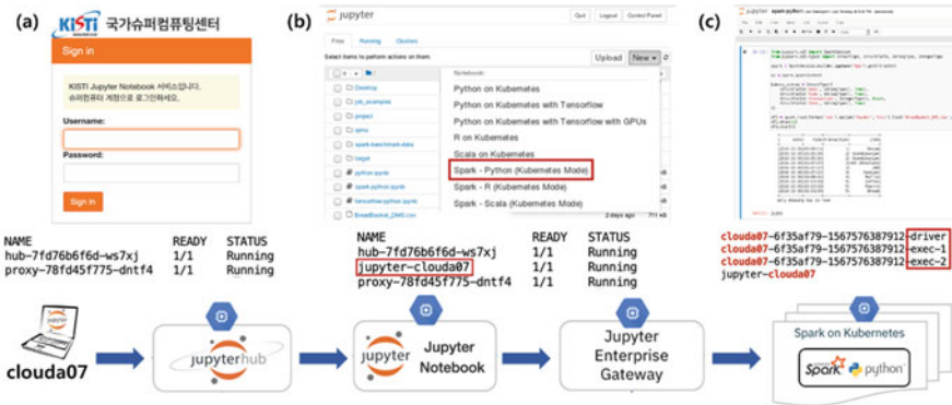
Fig. 3 Use case scenario of a container-based web interface for big data analysis using spark
