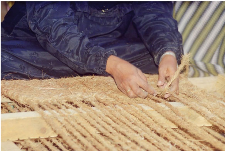
Fig. 83 Weaving a camel bag from date palm coir using a loom, Fayoum, Egypt
