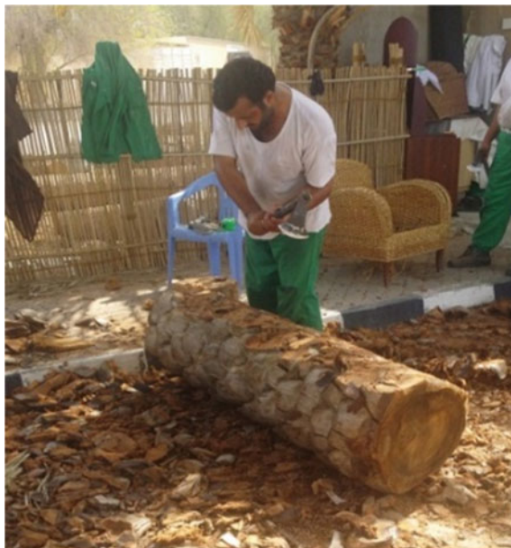
Fig. 93 Peeling and squaring a date palm trunk
