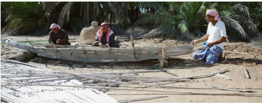
Fig. 38 Building a Shasha boat from date palm midribs
