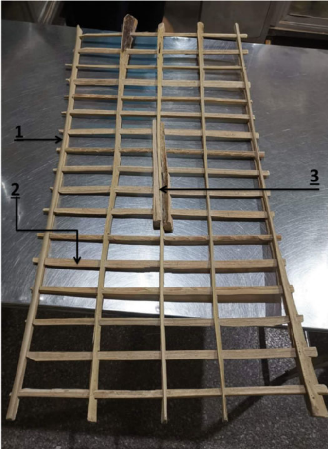
Fig. 27 Details of a date palm bread board. 1: the longitudinal members are cut to standard shapes and punctured at a specific spacing. 2: the transverse members are hammered through the punctured holes of the longitudinal members by friction. 3: additional members are added in the middle to prevent excessive deformation under the loads in the middle
