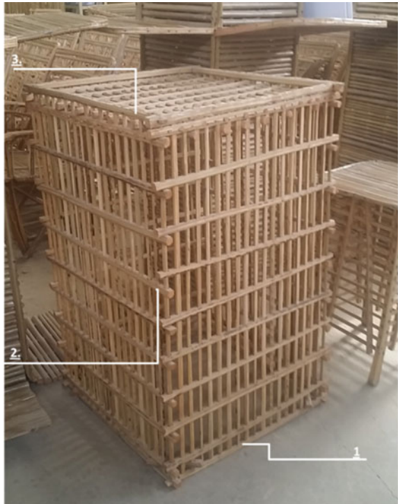
Fig. 26 Details of a standard date palm midribs chicken coop. 1: The vertical members are fixed through the holes of the bottom horizontal members at the base. 2: Secondary pre-punctured horizontal members are driven down to tie the vertical members. 3: The vertical members are leveled by the top horizontal members
