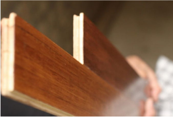
Fig. 9 Parquet pieces from palm midribs before assembly to satisfy a demand of flooring 120 m 2
