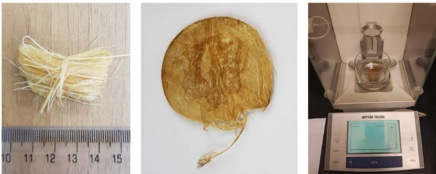
Fig. 11 Density samples preparation and measurement (Elseify et al. 2018)
