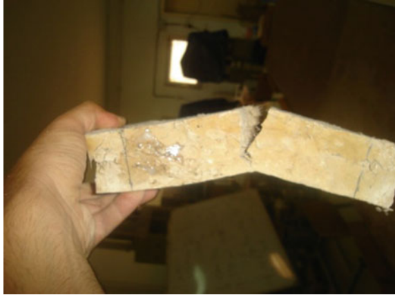
Fig. 11 Flexural failure of date palm reinforced adobe clay bricks
