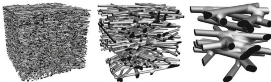
Fig. 4 Illustration of the correlations between pore size and fiber diameter at a constant porosity of 80% in a fixed volume (Ma et al. 2011)
