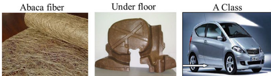
Fig. 3 Under floor protection trim of Mercedes, A-class made from abaca fiber reinforced composites (Faruk 2006)
