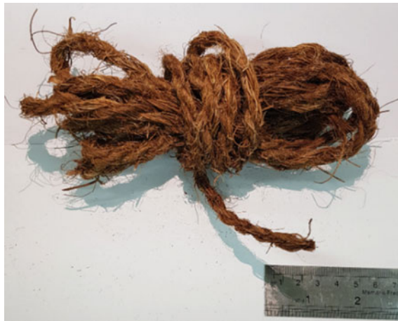
Fig. 2 A hand-made two-ply yarn from DPF
