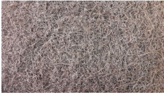
Fig. 12 A needle-punched nonwoven fabric from DPF
