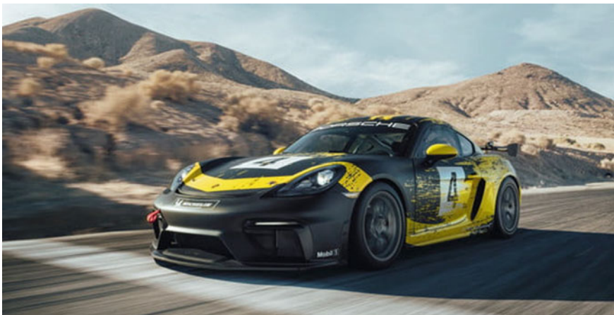
Fig. 4 Porsche 718 GT4 sports car made from natural-fiber (hemp & flax) composites
