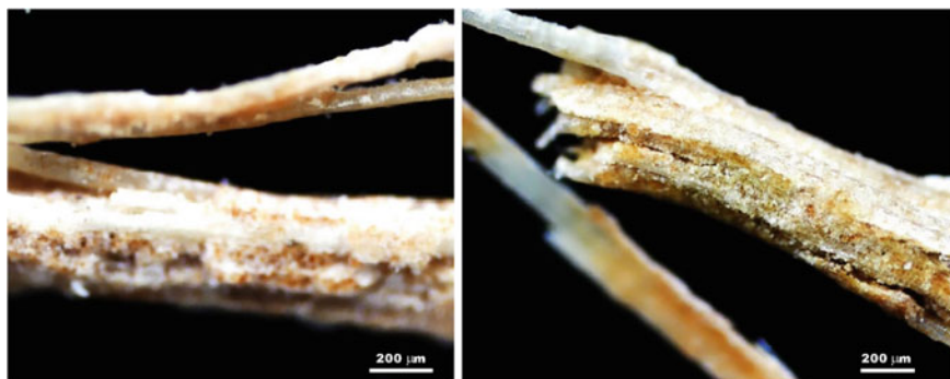
Fig. 6 SEM morphology for untreated Date palm fiber
