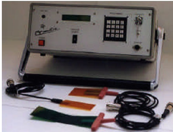
Fig. 15 The thermal conductivity measuring device CT meter
