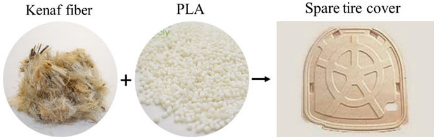
Fig. 4 Spare tire cover made from kenaf fiber reinforced PLA composites for Toyota RAUM ( https://www.slideserve.com/vincent/man-made-cellulose-fibres-as-reinforcement-for-poly-lactic-acid-pla-composites )
