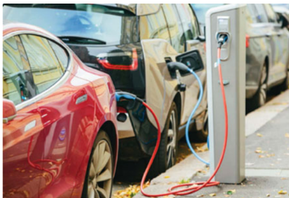
Fig. 18 Level two charging [16]. Source Arthur D. Little
