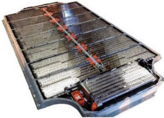
Fig. 15 Battery pack of Mitsubishi [14]. Source Mitsubishi
