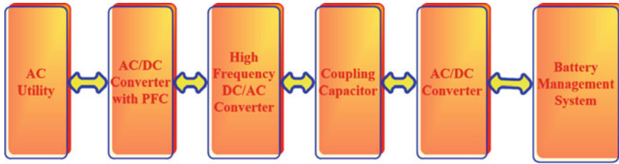
Fig. 6 Diagram of Capacitive contactless charging (CCC)
