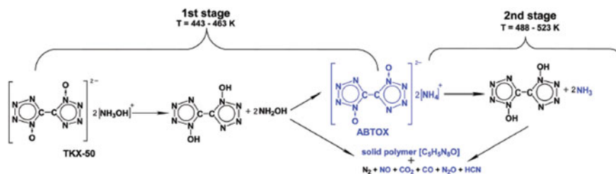
Fig. 38 Proposed mechanism for the two-stage thermal decomposition of TKX-50 by Muravyev et al. in which ABTOX is formed as an experimentally detected intermediate (indicated in blue) (Muravyev et al. 2017). Reproduced with kind permission from the publisher from Muravyev et al. (2017)
