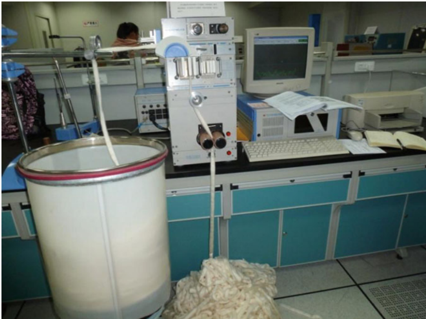
Fig. 6.6 Evenness testing system, image taken by Dr. Muhammad Qasim Siddiqui at Donghua University, China
