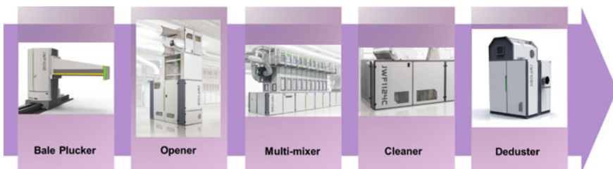
Fig. 9.1 The flow of blowroom machines
