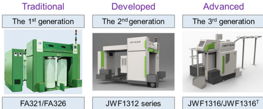
Fig. 9.21 The development of drawframe of Shenyang Hongda Textile Machinery Co., Ltd
