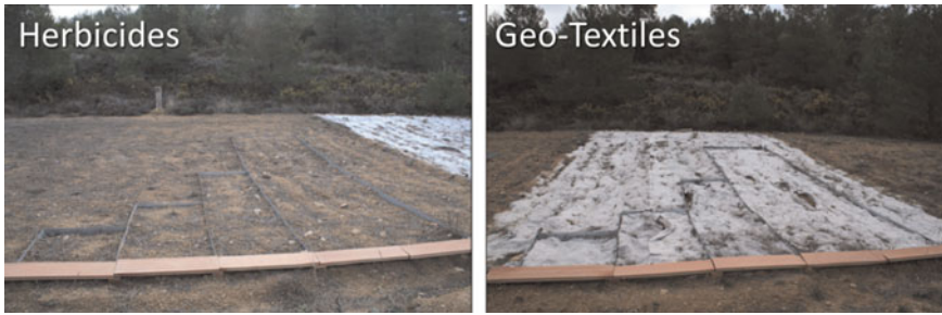
Fig. 12.13 The illustration of land protection by herbicides versus geotextiles [17] (Fig. 1 on page 211) Copyright © 2010 John Wiley and Sons, Ltd
