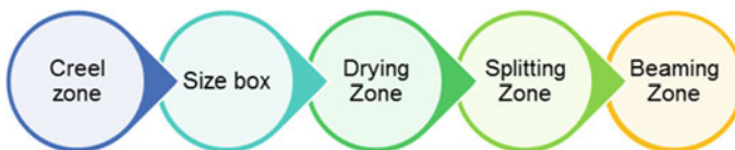
Fig. 10.5 Block diagram of sizing machine
