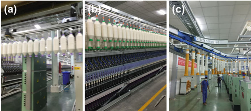
Fig. 8.5 The roving bobbin transport system in a cotton spinning industry in Uzbekistan, a roving bobbins automatically being transported from simplex to ring frame, b roving bobbins has been installed to ring frame, and c empty roving bobbins automatically being shifted from ring-spinning frame to simplex
