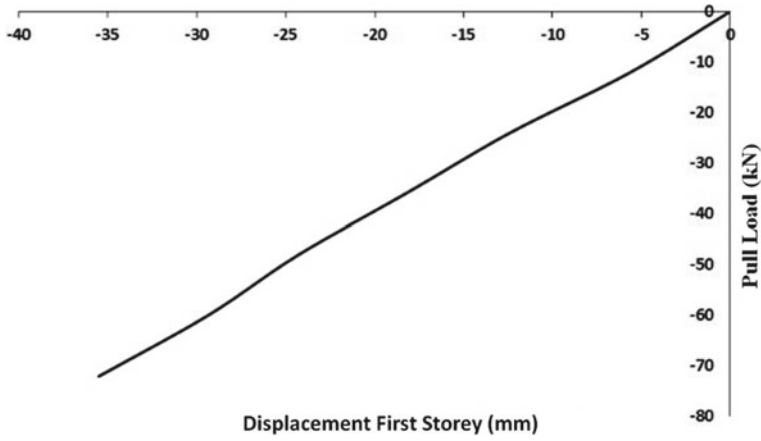
Fig. 25 Load—displacement for bottom storey (pull) of experimental frame
