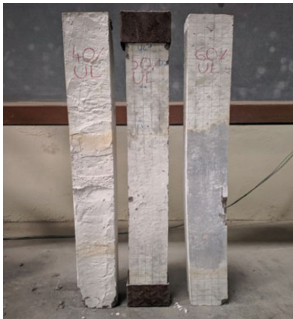
Fig. 10 Samples of failure pattern for column
