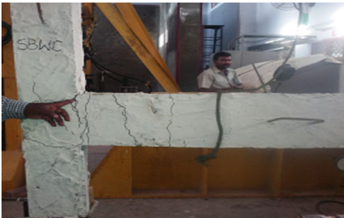
Fig. 9 Cracking pattern of beam–column joint SBWC
