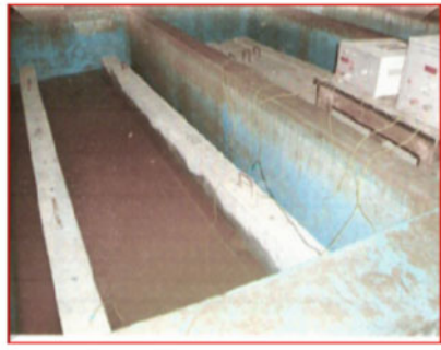
Task 2: Induction of corrosion / Accelerated corrosion process
