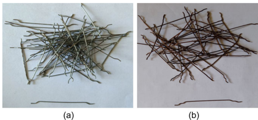
Fig. 1 Appearance of hooked end steel fibres a 3D and b 5D
