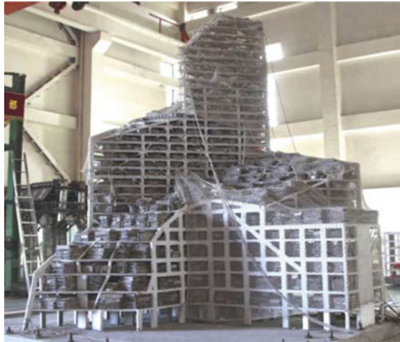
Fig. 3 1:20 scaled model of an irregular high-rise RC structure [23]
