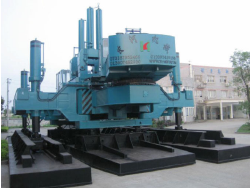
Fig. 1 High capacity of jacked-in machine (Google image)
