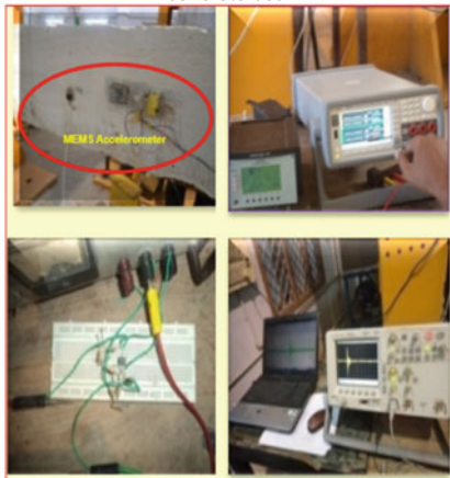
Task 5: Acquire information using necessary instrumentation in the concrete beam specimen and Data Acquisition
