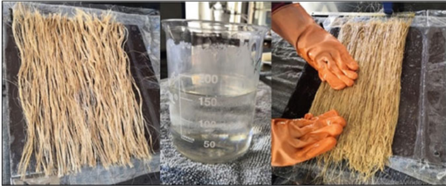
Fig. 6 Fabrication of BFRC using banana fibre and epoxy-hardener mixture
