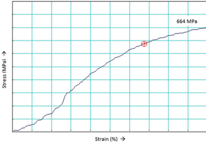
Fig. 5 Stress versus Strain diagram for T1—Annealed sample which is having fine interlamellar spacing
