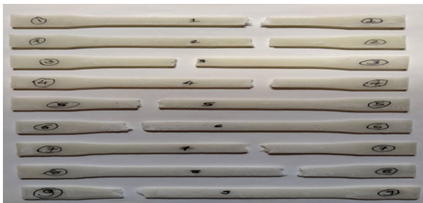
Fig. 5 Specimens after tensile test
