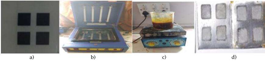
Fig. 2 a Phototool, b 3D exposure unit, c 3D etching unit, d finished component
