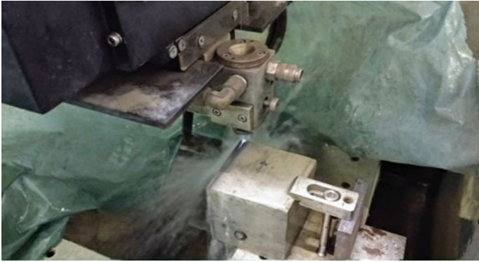
Fig. 2 EDM wire cutting
