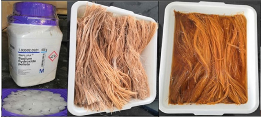
Fig. 5 Chemical treatment of banana fibre using 1% NaOH solution
