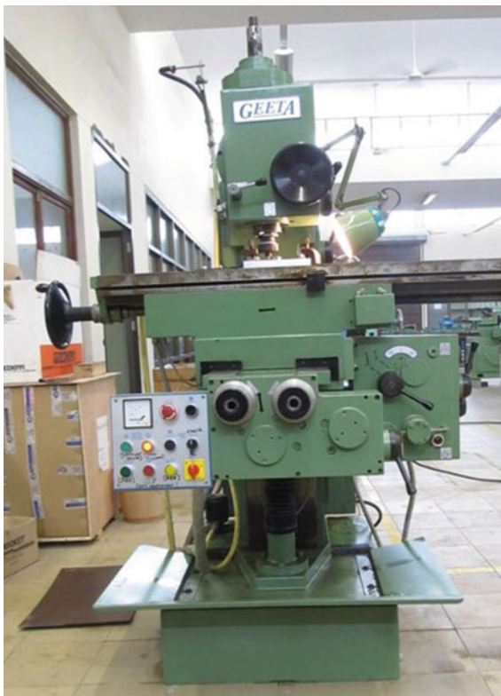
Fig. 1 Modified vertical milling machine employed for FSW
