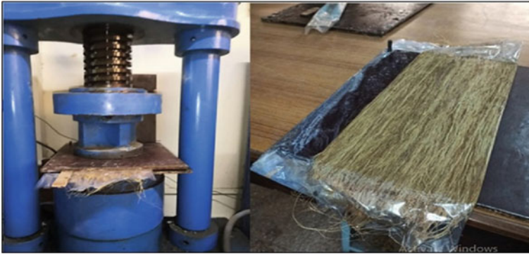
Fig. 7 Compression of composite sheet using compression press
