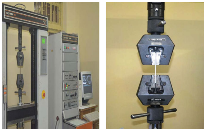
Fig. 2 Experimental setup for tensile testing on UTM
