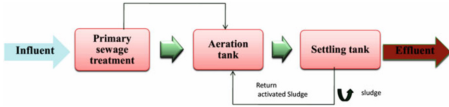
Fig. 17.2 Flow chart showing activated sludge process
