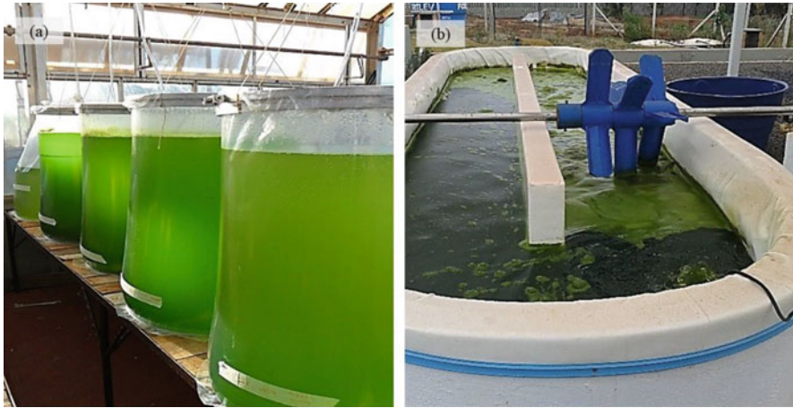
Fig. 23.3 (a) Transparent tubular photobioreactor for the cultivation of microalgae aiming inoculum production and (b) open tank
