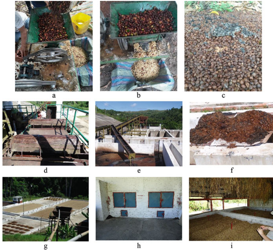
Fig. 21.2 Coffee processing: semi-dry (a–c) and wet method (d–i)
