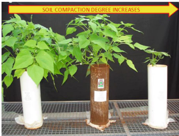
Fig. 22.6 PVC columns with common bean cultivar IPR Eldorado cultivated in a clayey Dystropheric Red Latosol (51 dag kg -1 clay) submitted to degrees of soil compaction in a subsurface layer of 10–25 cm depth. From left to right: Degree of compaction = 60% (Soil bulk density = 1.0 Mg m -3 ); 78% (Soil bulk density = 1.3 Mg m -3 ) and 90% (Soil bulk density = 1.5 Mg m -3 )
