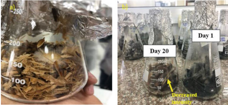
Fig. 11.10 SSF system: (a) presence of mycelium during the growth of Pleurotus djamor (Pd318) in sugarcane bagasse; (b) oxidation of textile dye A19 in a solid medium
