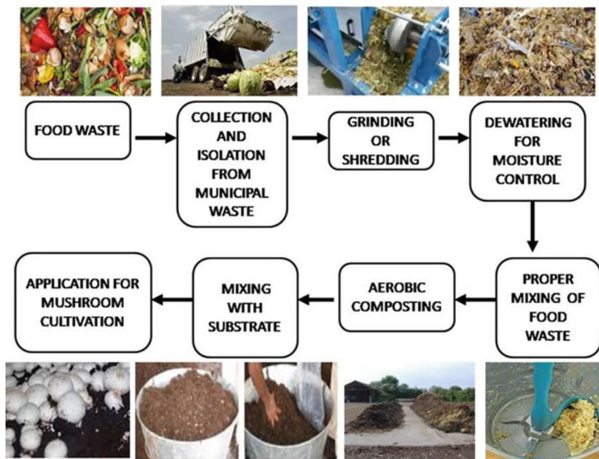
Fig. 17.2 Processing of food waste into compost and further, its use in mushroom cultivation. Compost is mixed with substrate for mushroom cultivation
