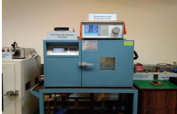
Fig. 8.11 Two pressure humidity generator (Thunder Scientific 2500) along with chilled mirror hygrometer (RH 370) established at CSIR-NPL
