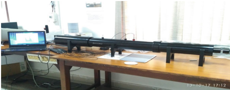
Fig. 8.25 Impedance tube facility at CSIR-NPL
