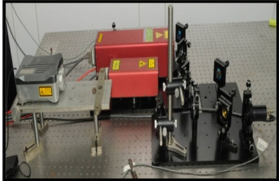
Fig. 7.12 Iodine stabilized He–Ne laser
