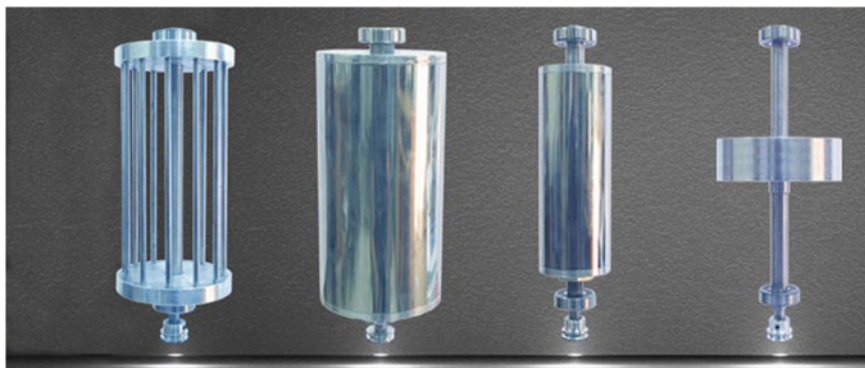
Fig. 2.13 Different configurations of cylindrical or disc type collectors. Adapted and reproduced from Ref. [141]
