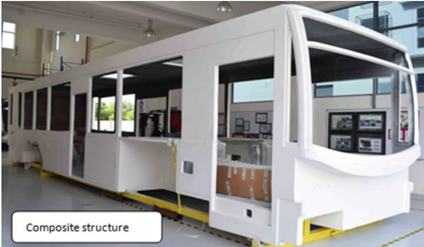
Fig. 1 Composite monocoque chassis (with permission from Sync R&D Sdn. Bhd.)
