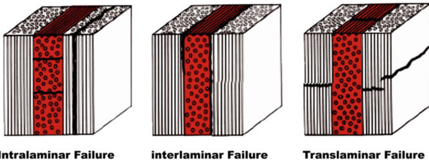
Fig. 8 Failure mechanisms in 0/90/0 laminate
