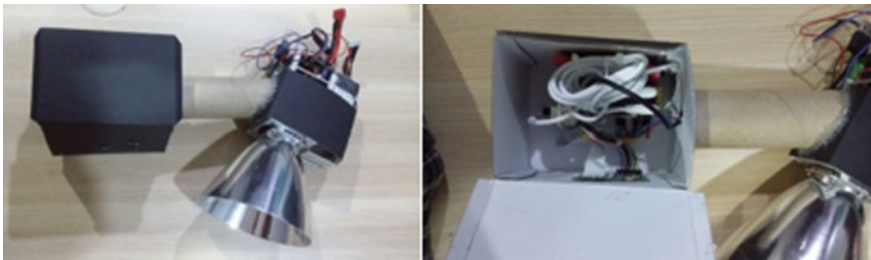
Fig. 18 Various view of the thermal camera prototype
