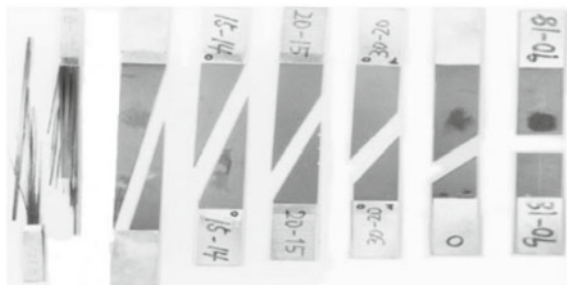
Fig. 7 Fatigue of tensile coupon specimens at room temperature [25]
