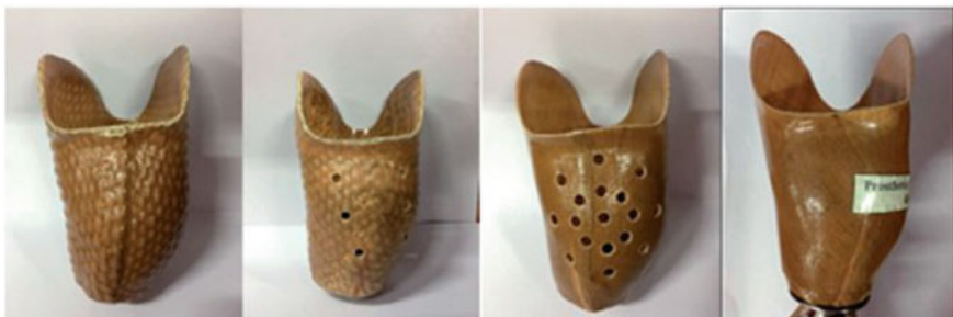
Fig. 12 Natural fiber socket [29]
