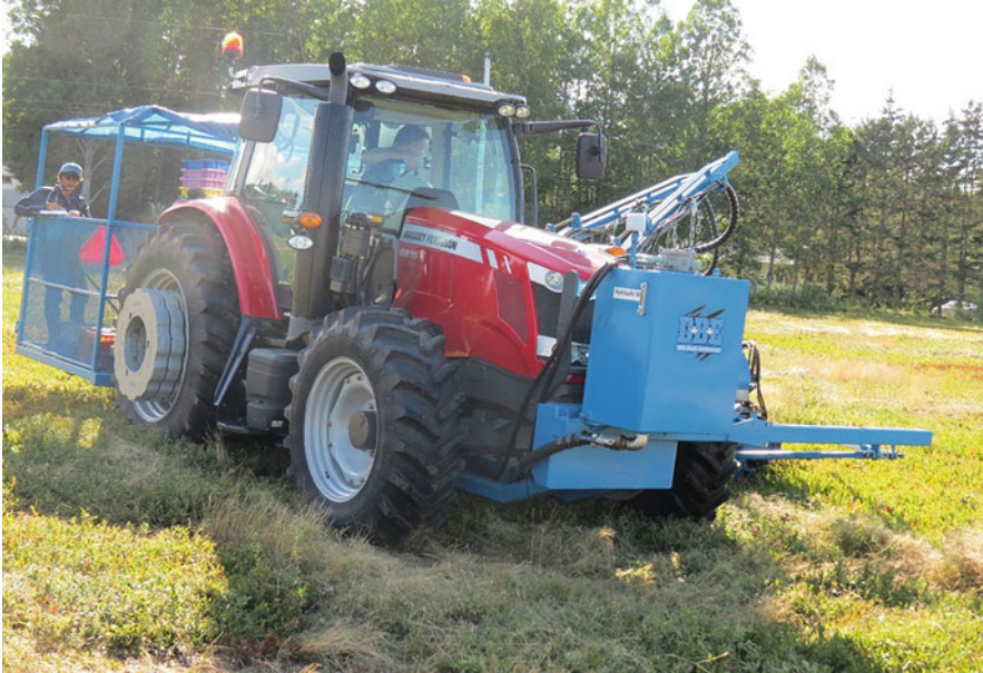
Fig. 21.1 Profit from a farm business is needed to purchase innovative farm equipment, such as tractors and harvesters. This picture illustrates a new labour-saving harvester for lowbush blueberries
