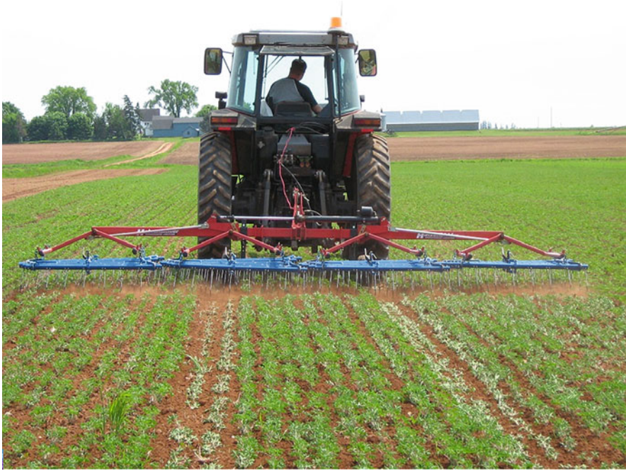
Fig. 20.7 Mechanical weeding equipment such as this tine weeder allows weed control after the crop has emerged without the use of herbicides. (Photo credit: A. M. Hammermeister)
