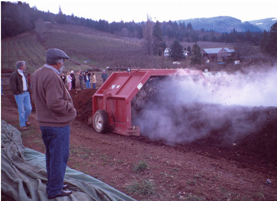
Fig. 8.5 Turning a large-scale commercial compost windrow in Oregon, USA. This compost is used to fertilize a local orchard. (Picture from Washington State University extension service)
