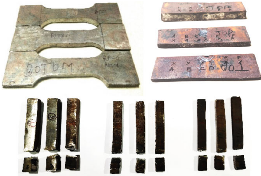
Fig. 3 Pictorial representations of a Tensile Test; b Hardness; c Izod Specimens
