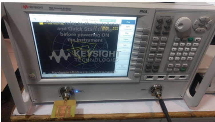
Fig. 15 Measurement setup of Input Impedance at 7 GHz
